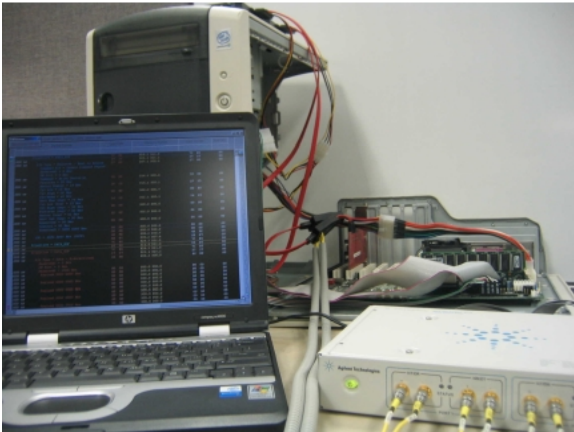
Fig. 9: SATA gen2 Protocol Trace Capture Using Analysis Probe
