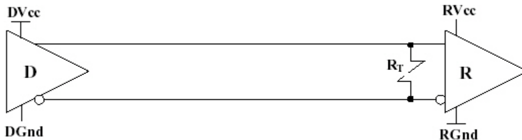
Fig. 6: Typical LVDS Termination Technique Using Internal Failsafe
