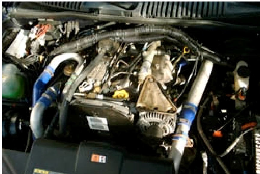
Under the hood, a 2.5-liter diesel, and a 37-kW electric motor
